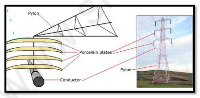
electricity .They do not melt when a high current flows through them as they have high melting and boiling points. Hence they are used in high voltage electricity towers to keep the wires from touching the pylons or from touching each other.
